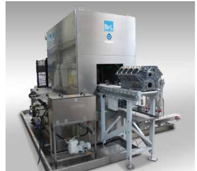
Version: NiagaraDFS with synchronised flow-through process for optimising cycle times
