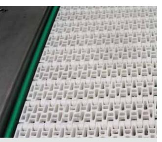
**Plastic conveyor** for sensitive component surfaces
