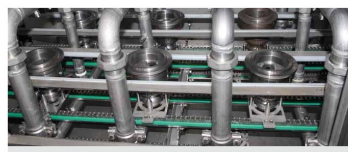
**Chain conveyor** for similar parts without workpiece carriers or for parts on (screw fixed) workpiece holders or in baskets
