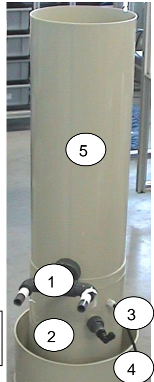
Pump station with foam tower
