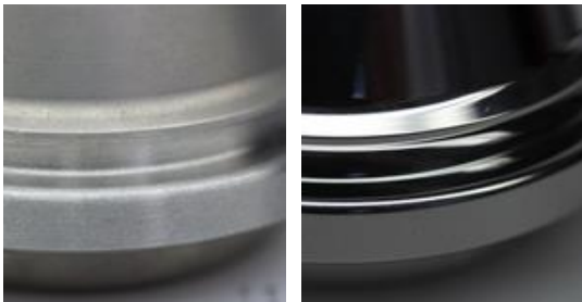
Forming surfaces of the can seamers before and after OTEC finishing
