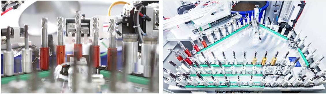
Automatic tool change with chain loader
