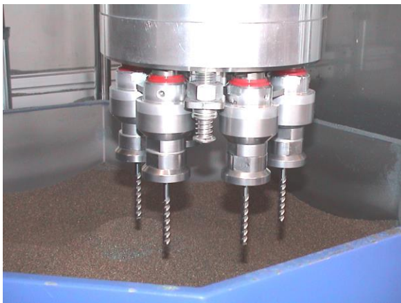
Fig.: Tool holder with workpieces just before immersion in the process container.
