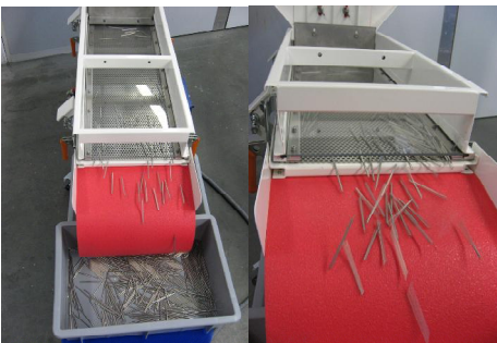
Picture 2 and 3: new device as addition to the Unisepa for the separation of long, thin workpieces
