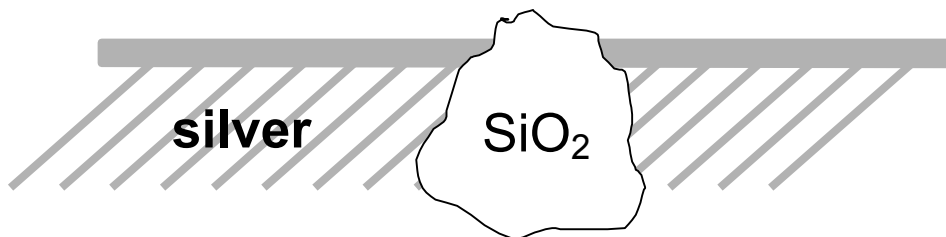
Figure 7.1 Embedded SiO 2 particle
