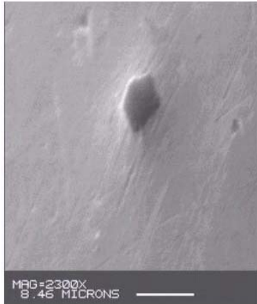
Figure 7.3 “Comet tails” after final polishing
