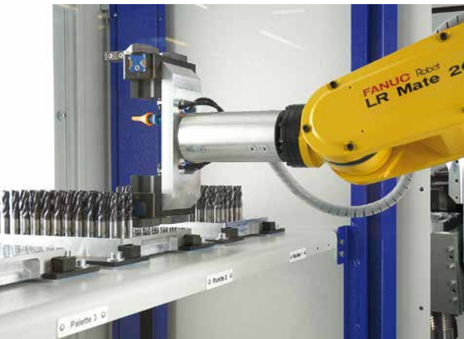
A robot arm grabs a milling tool from the workpiece pallet
