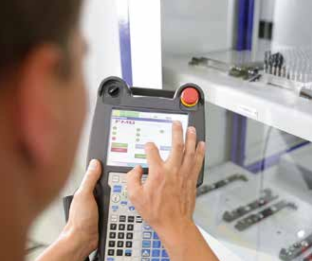
Touch panel for controlling the robot arm on the SF RLS
