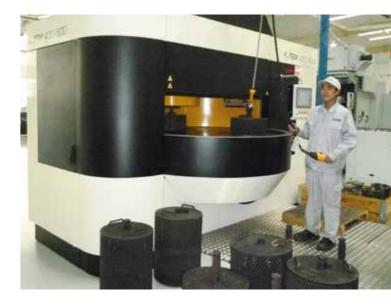
Shandong Changlin is a manufacturer of construction and agricultural machines and diesel engines. The versatility of the thermal deburring machine from ATL allows for such a range of products.
