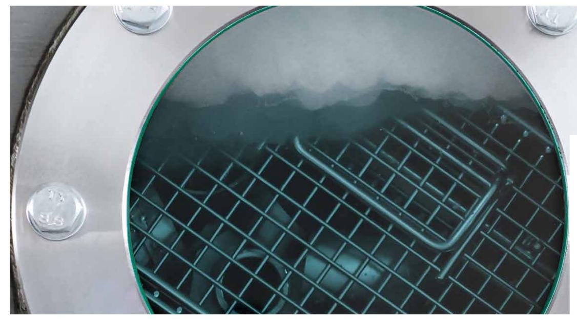
After the TEM process, the burnt material deposits in the form of ferric oxide on the whole surface of the workpiece. Due to this fact, a subsequent treatment of the components is gene-
