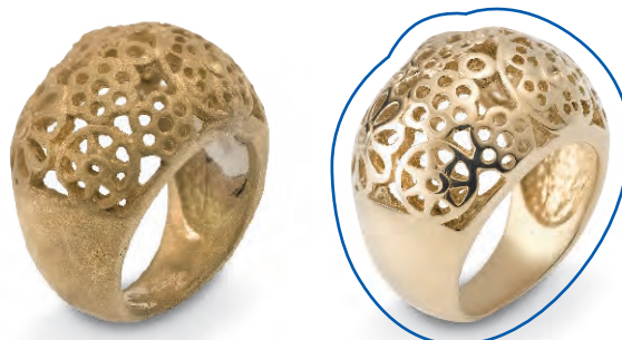
Electropolishing guarantees perfect surfaces even in the smallest gaps.
